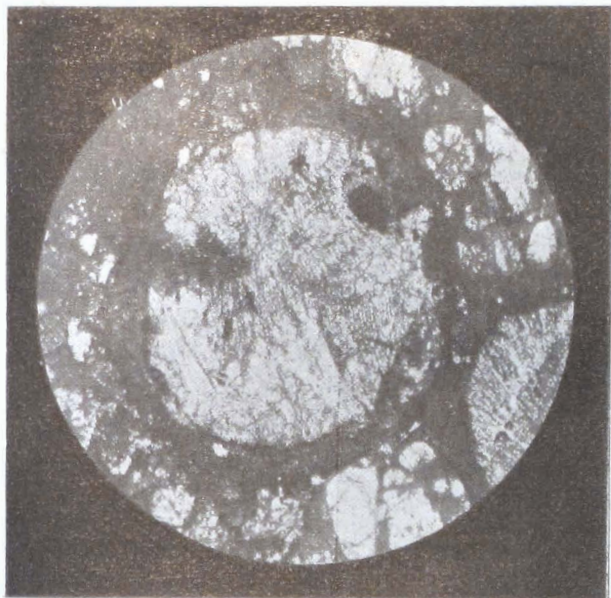
FIG. 1.—Chondrule of enstatite from the Khohar meteorite, showing a rim of metallic iron \times 32 .
